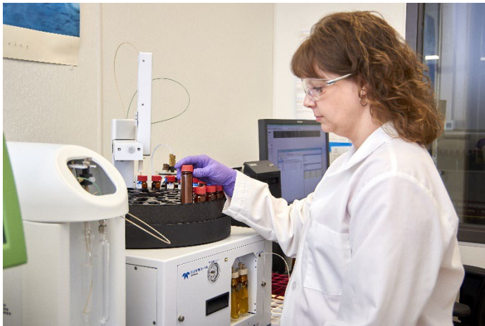
Technician operating GC/MS equipment at the Kanawha Valley Treatment Plant
