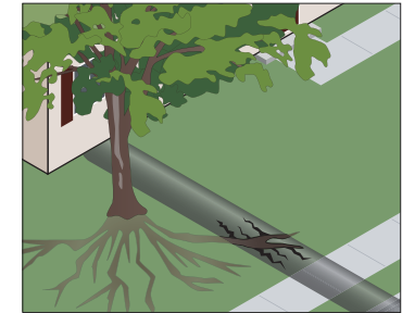
Root invasion A partial or complete blockage of the sewer service line by tree roots.
