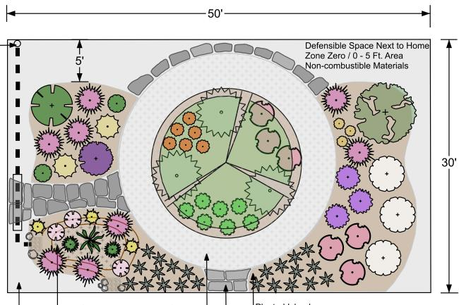
Rain Garden with 3" Depth of Salt & Pepper Pea Gravel in Bottom to Ensure No Ponding for Mosquito Control with Cobble & Boulders at Inflow & Outflow
