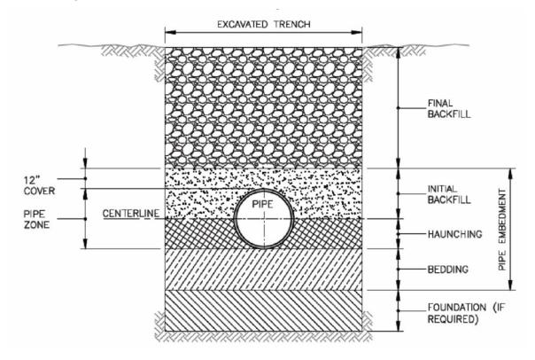
A. Foundation – A foundation is necessary only when native soils are unstable. For such conditions, the trench is over-excavated and a layer of supportive material is placed and compacted to provide a firm foundation for the subsequent pipe embedment materials. Must be approved by the OWNER prior to over-dig.
