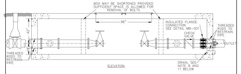
1. VAULT WALLS AND ROOF TO BE OF CONCRETE.
