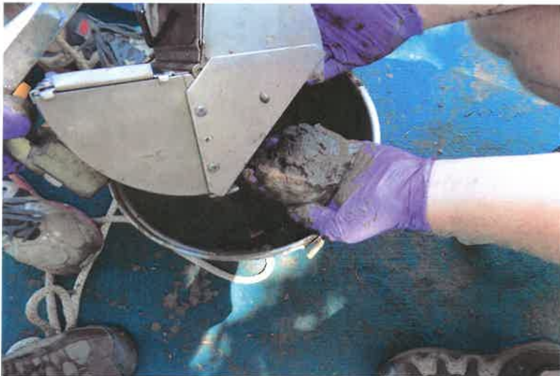
Photo 9: Removing Sediment from Petite Ponar into Metal Bucket
