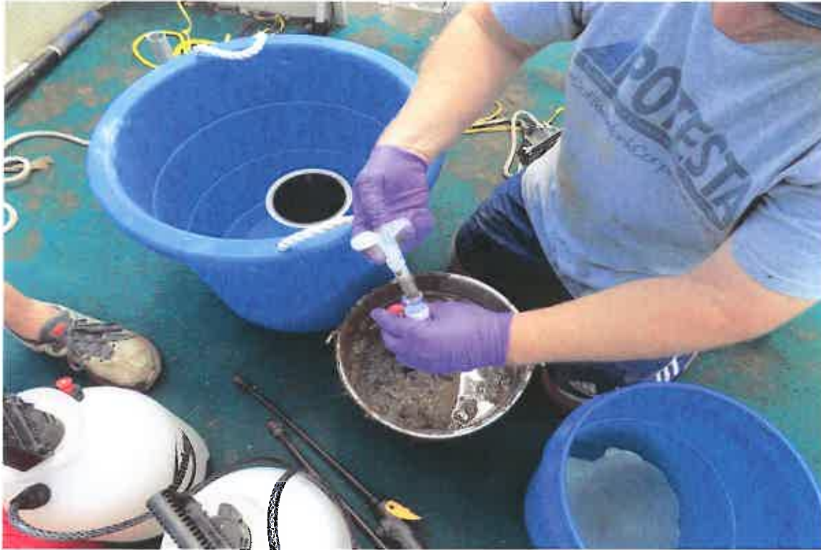
Photo 18: Placing Sample from Terra Core™ Sampler into 40 mL Vial
