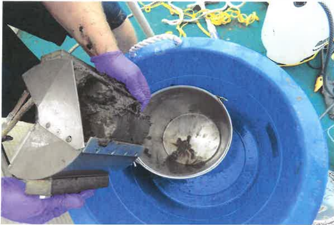
Photo 10: Removing Sediment from Petite Ponar into Metal Bucket
