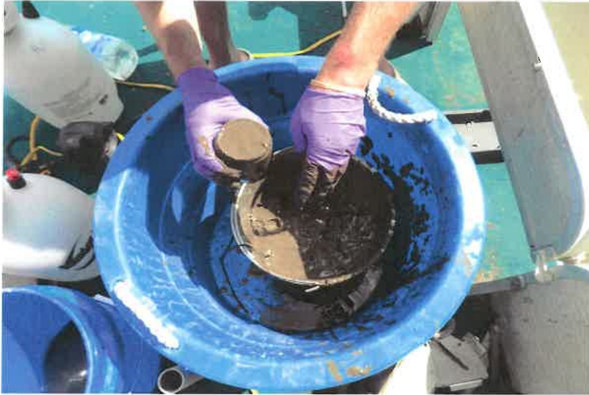
Photo 20: Sediment Placed in 8-ounce Glass Soil Jar
