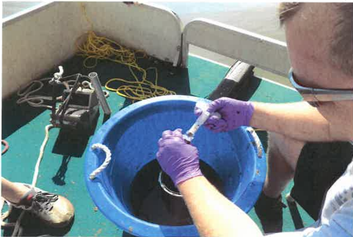
Photo 17: Placing Sample from Terra Core™ Sampler into 40 mL Vial
