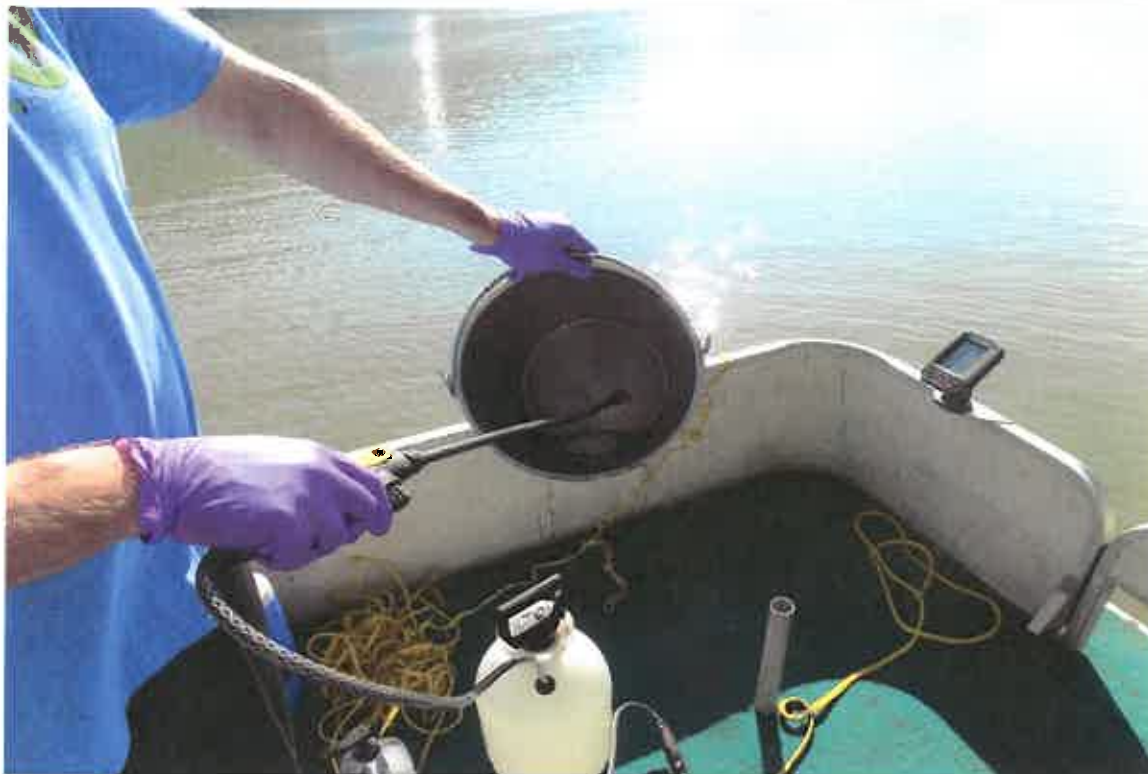
Photo 12: Decontaminating Steel Bucket with Liquinox® Water Solution
