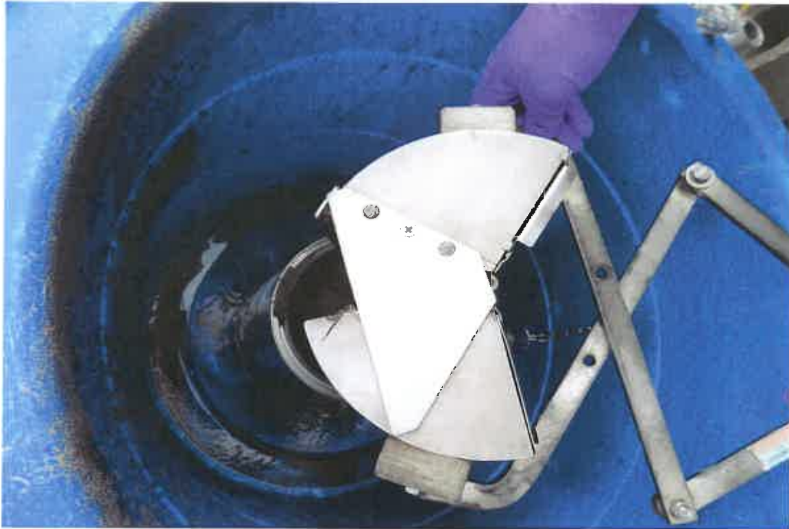
Photo 8: Removing Sediment from Petite Ponar into Metal Can
