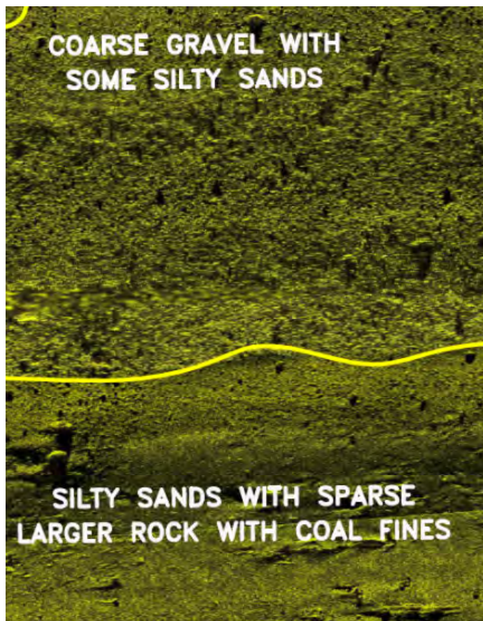
Figure 8: Varied imaging due to the differing sediments.
