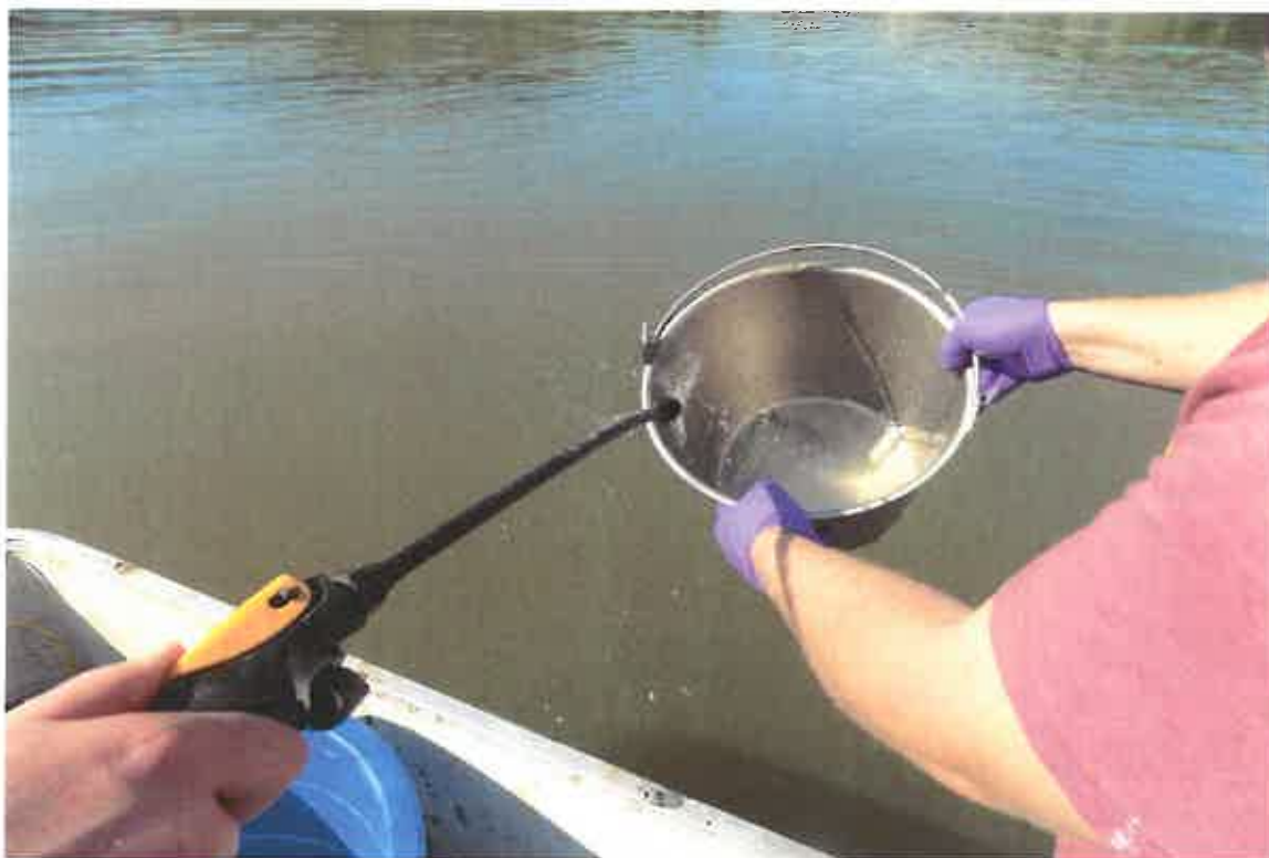
Photo 13: Decontaminating Metal Bucket with Liquinox® Water Solution
