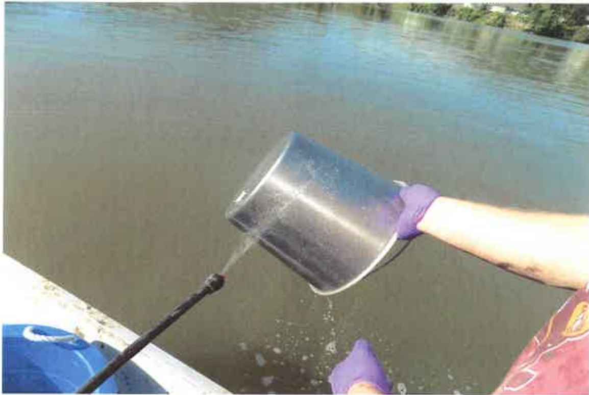
Photo 14: Decontaminating Metal Bucket with Liquinox® Water Solution
