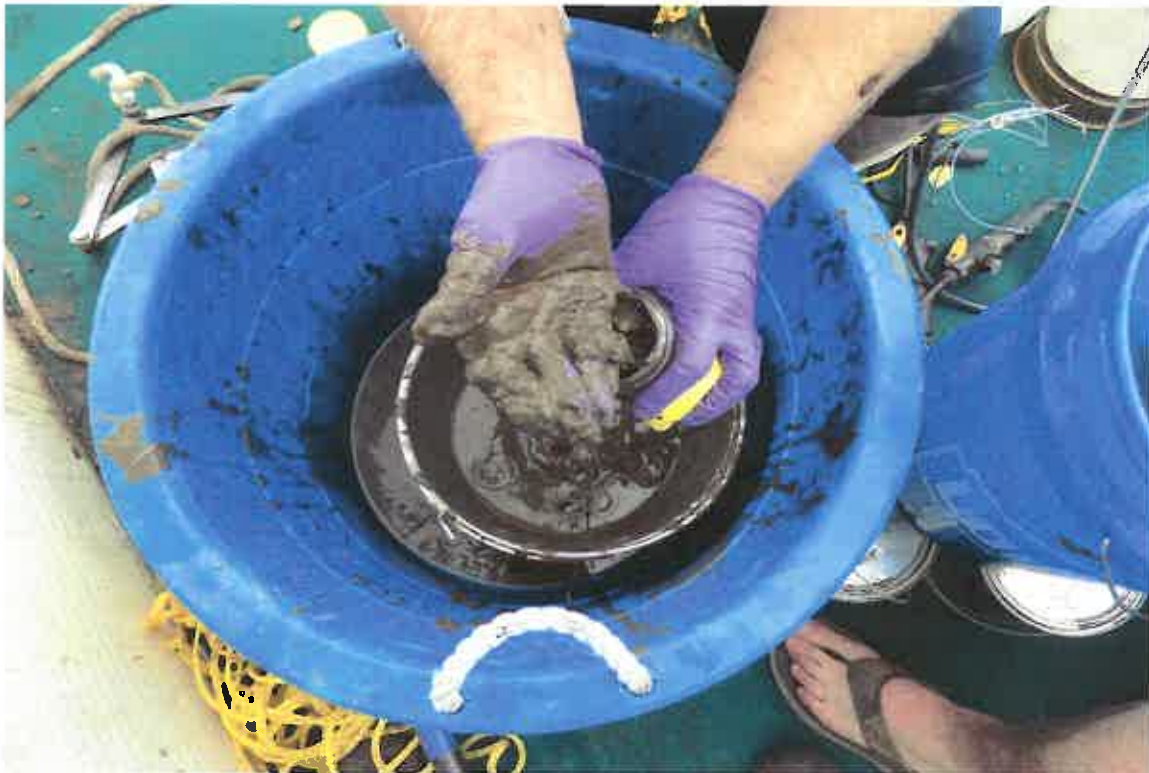
Photo 21: Sediment Placed in 8-ounce Glass Soil Jar from Metal Bucket
